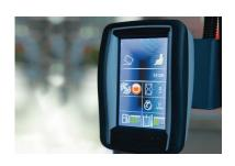
The standard high-resolution color display shows all relevant operating information. A built in service timer automatically notifies when Preventative maintenance is due preventative less downtime.
