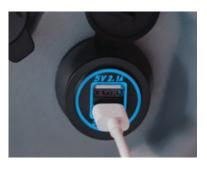
Operator safety is paramount. A USB connection at the steering column allows the operator to keep their mobile device charged in the event of unforeseen circumstanes or an emergency.
